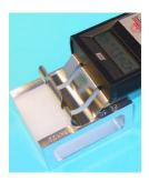
The test module PE30 is used for testing the accuracy of the DM4A moisture meter for wood and moisture measurements for building moisture measurements
