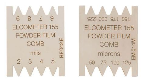
The Elcometer 155 is designed to measure uncured powder coating film thickness. This enables the application system to be set up and fine tuned prior to the curing process. In turn, this will reduce the amount of scrap and over-spray.
