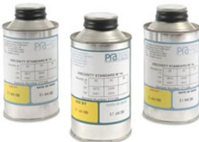
Silicone standard oils are used to check viscosity measurements. The values are given for 6 different temperatures between 20°C and 27°C
