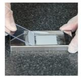
2. Using the plastic scraper, scrape over the coating allowing the excess to fall into the overflow chamber. Allow the coating to dry.
