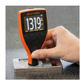
3. When fully cured, calibrate a ferrous coating thickness gauge on the side of the CCM then measure and record the dry thickness at the centre of the coating.
