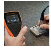
4. Measure the same point using the Elcometer 500. Enter the dry film thickness measurement and save it in the Elcometer 500's Coating Materials list.
