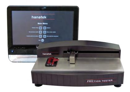
The Advanced Friction Tester produces detailed fingerprints of new substrates, coatings and production samples. These characteristics can be saved and compared at any time allowing the manufacturer specify the optimum surface finish for any packaging process.
