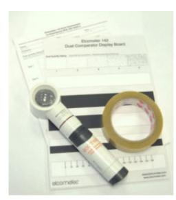
The Elcometer 142 ISO 8502-3 Dust Tape Test kit allows assessment of the quantity and size of dust particles on surfaces prepared for painting.
