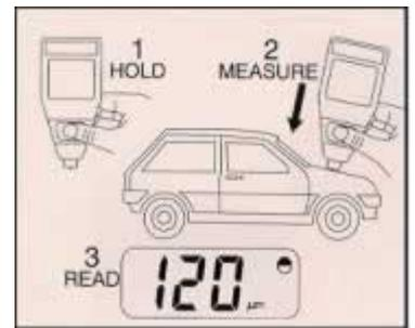
**Why do some paint jobs "feather" or build from areas of low thickness to areas of higher thickness?** : Automobile companies tend to apply thin paint in areas with low chip potential and thicker paint in areas of high chip potential. The 311 will allow you to note that the paint can be thicker on the leading edge of the hood, rocker panels, and the lower sections of doors while being thinner on the trailing edge of the hood, roof, trunk, or any other area with low chip potential.
