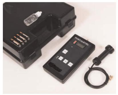
The Portalevel's accuracy and repeatability have been verified by First Article Tests (very stringent tests conducted on items for supply to the US military). They confirmed its accuracy as +/- 1.5mm. As well as accuracy, they also tested the robustness of the unit by dropping it three times to a metre and submitting it to varying temperatures. Following these stringent tests the US Navy purchased 100 units.
