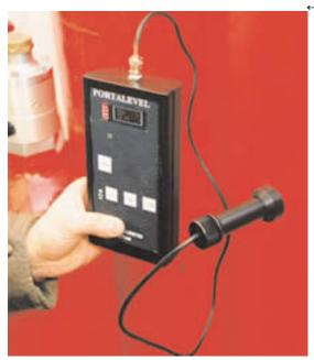
Magnetic Probe Sensor allows you to leave the probe on the surface and allow hands free operation
