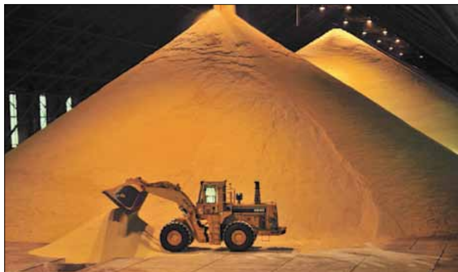
Raw sugar being poured into a QSL sugar bulk storage shed.
