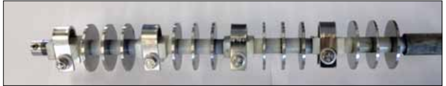
The specimen holder with three disk coupons and one U-bend coupon for each material. Photo courtesy of Sigrún Nanna Karlsdóttir.
