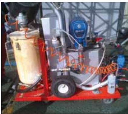
Graco Reactor EXP 2 Polyurea spray machine mounted on trolley for ease of transportation.
