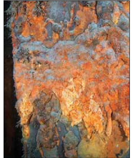
Figure 1: Damage caused to a material surface by microbiologically influenced corrosion.
