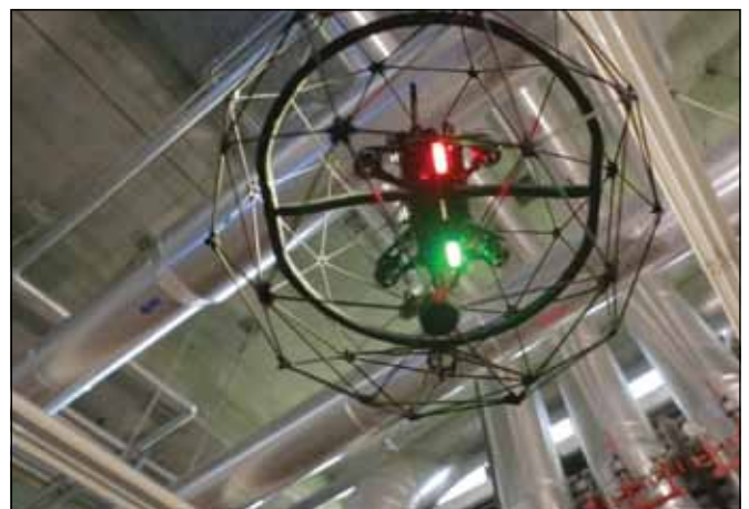
One marine consortium led by Robotica in Maintenance Strategies (RIMS) has proposed enclosing their drone within a protective cage.
