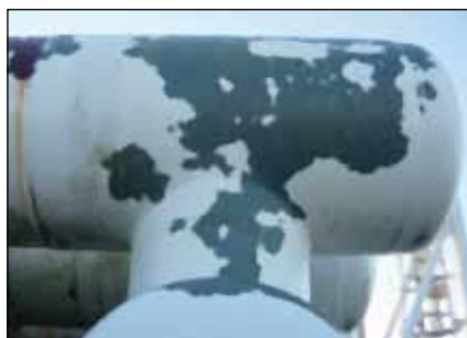
A white, polysiloxane topcoat delaminated adhesively from an organic zinc-rich primer on a pressurized vessel at a gas processing facility. Additionally, the coating system installed in the field-joint area delaminated to the bare steel (as shown in the upper left portion of the picture).
