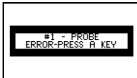
Figure 39. Example error message - no probe is connected to gauge
