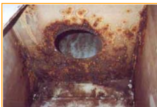
A ship's ballast tank is corroding after only 3 years in service
