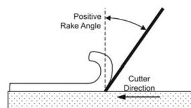
In the direction of travel, shown by the arrow, the cutter is angled behind the perpendicular to the surface at this point. It cuts the surface from the
