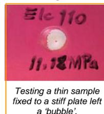
**Materials with a soft or an uneven surface** do not provide a stable surface for the tester. This results in a pull that is not at 90 degrees to the axis of the dolly or stub. A base support ring that is available with some models solves this problem. It is a metal disc with a central hole, its large area spreading the reaction force.
