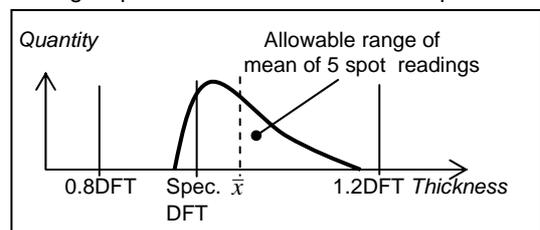
The thickness of the coating is acceptable if the DFT of an area fits within the curved part of the graph.
