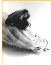
The ability to coat structures and ensure the adhesion is adequate is a requirement of some standards. For example, NORSOK 501 requires the bond strength in certain cases to exceed 5, 7 or 9MPa rather than achieve a particular figure (See *Elcometer 109, left*). In this case, it is not necessary to test to breaking point.
