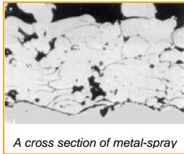
the spray still hot when it lands on the surface or the layer will easily disbond. Because the coating is porous, the test adhesive must have a high viscosity, or it will penetrate through the layer, possibly to the substrate, giving a higher and inaccurate reading.
