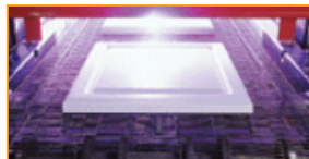
UV curing of wooden doors
