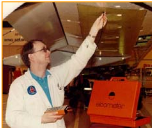
Testing the coating on a wing with the Elcometer 355 Top Coating Thickness Gauge
