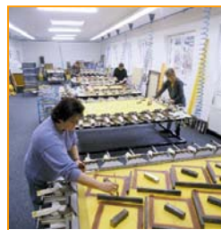
Emulsion thickness confirmed, the mesh is ready for framing
