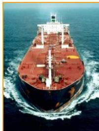
These huge steel vessels are continuously under attack from the conditions they operate in. The high salt content of the sea leads to aggressive corrosion on the outside, while the cargo of warm crude oil corrodes from the inside. It is therefore necessary that the protective coatings applied to the tanker are of the correct thickness and that regular checks are made
