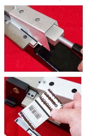
5.0 Remove the cut sample from the side of the sample cutter.
