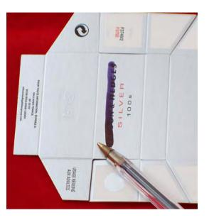
2.0 Remove excess material so that the carton fits in the sample cutter
