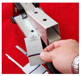
5.0 Place the sample in the cutter with the test crease along the line.
