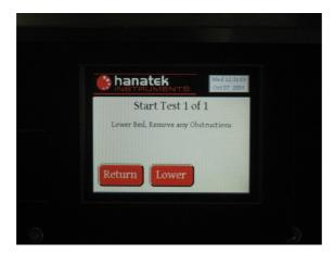
If the plane is raised ensure the lowering area is free from obstructions. Press "Lower" or the green button to proceed.
