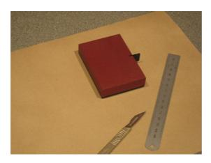
**Bed Sample-** Cut a sample with a width of 70mm-100mm and between 80-180 mm long, hold it in place with the small magnets.
