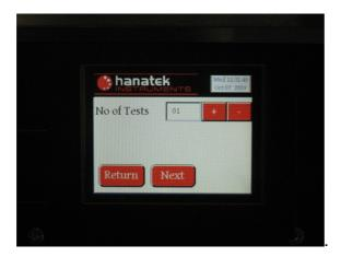
Use the +/- to select the number of repeat tests required. Press the "Next" to proceed to test screen
