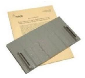
The Elcometer 999 Surface Weld Comparator provides for the first time, a means of comparing the quality of welds.
