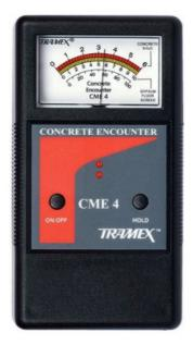
The CME4 is for measuring moisture content instantly in concrete floors and floor screeds without the need to drill or damage the surface up to 20mm into the substrate. This non-destructive analog moisture meter is ideal for concrete floors and slabs providing instant and precise quantitative measurement of moisture content using Gravimetric testing as a baseline.
