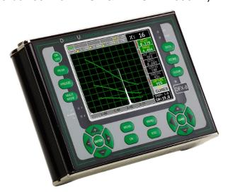
The Dakota FX80 Bench Top Ultrasonic Flaw Detector is available in two models: Dakota FX80-DL Bench Top Flaw Detector and Dakota FX81-DL Bench Top Flaw Detector. The time corrected gain (TCG) feature automatically compensates for sound attenuation through a material, further increasing the performance of the gauge.
