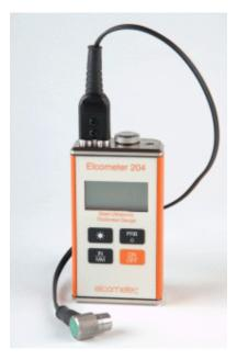
The Elcometer 204 Steel Ultrasonic Thickness gauge is a handheld gauge providing fast and accurate measurements of the thickness of steel. The principal advantage of ultrasonic measurement over traditional methods is that ultrasonic measurements can be performed with access to only one side of the material being measured.
