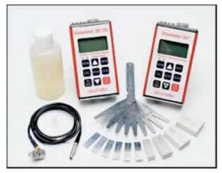
The Elcometer 207 series of precision ultrasonic thickness gauges are designed to provide accurate measurements on thin materials. Using the latest transducer designs - the single element delay tip transducer - the Elcometer 207 gauges will measure thin materials in "Echo-to-Echo Mode" and then automatically switch to "Interface Echo Mode" when measuring thicker materials and plastics.
