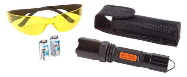
The Elcometer 260 UV Pinhole Flashlight is battery powered and housed in a rugged aluminium case providing a quick, low cost method of testing coatings for pinholes. Featuring a three-Watt purple light emitting diode, the Elcometer 260 UV flashlight has a beam wavelength of 405nm (±5nm), which the human eye perceives as a purple light.
