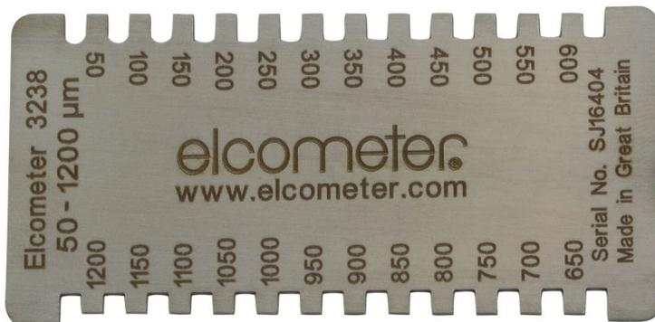
These stainless-steel combs are wire eroded to provide an accuracy  $\pm 5\%$  of marked value or  $\pm 3\mu\text{m}$ , whichever is greater, and are supplied with either Metric or Imperial measurements.
