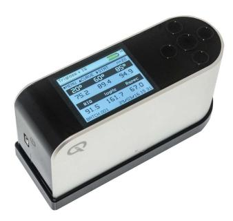
The Elcometer 408 provides the very latest in gloss measurement technology, providing accurate gloss, haze and distinctiveness of image (DOI) analysis in a single reading.
