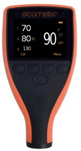
The Elcometer 456 Industrial Protective Coating Thickness Gauge<sup>1</sup> is designed to measure dry film thickness on shot or grit blasted steel substrates.
