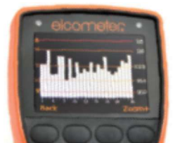
Individual batch readings can be reviewed numerically or graphically
