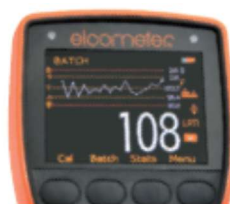
On-screen trend graph displaying last 20 measurement values
