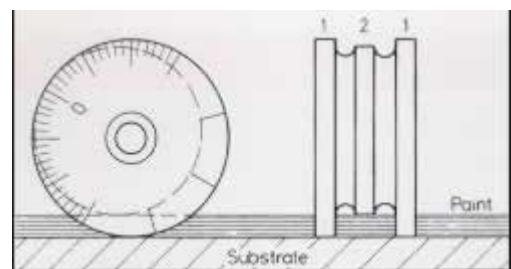
Roll the wheel through the wet film with the side 1 in the diagram touching the substrate. Roll for at least one whole turn and slowly enough for wetting to occur. Roll the wheel backwards by at least one complete turn. The wet film thickness is read from the scale, at the end of the wetted segment of the middle circle, 2 in the diagram
