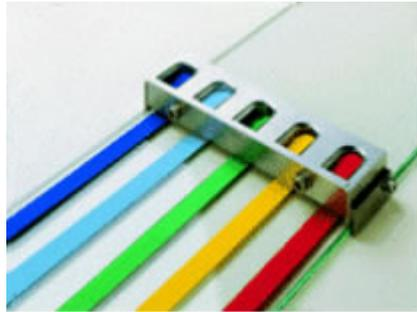
Made of hardened stainless steel with a bevelled flat-edged blade, these applicators apply films 12mm wide. Generally on any flat and firm surface and especially on glass for evaluation of drying time.
