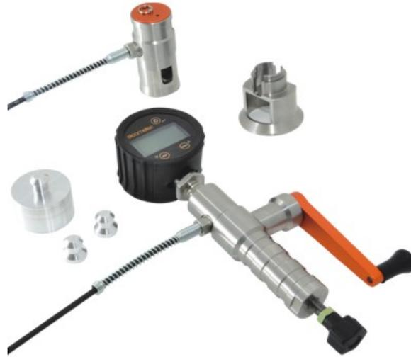
The **Elcometer 506 Adhesion Testers** are lightweight, portable and easy-to-use adhesion gauges available in analogue or digital versions and are suitable for measuring the pull-off adhesion of coatings up to 50MPa either on-site, or in the laboratory.
