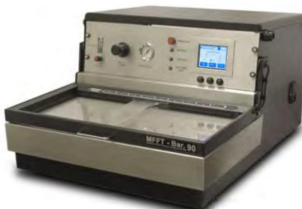
The Rhopoint MFFT is the industry leading instrument for measuring the minimum film forming temperature of water based materials. Definition - "MFFT is the lowest temperature at which a latex, emulsion or adhesive will uniformly coalesce when laid on a substrate as a thin film." An accurate MFFT value allows the formulation of products that cure correctly under specified application conditions.
