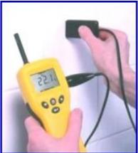
**Condensator Mode** A specialised hygrometer mode for assessing the risk -or confirming the presence -of condensation on surfaces. When the Surface Temperature Sensor is connected and held against a surface, the MMS displays the difference between the surface's temperature and the dew point, together with text messages that confirm whether or not condensation is occurring. An optional infra red remote surface temperature sensor can also be used for rapid condensation risk analysis.
