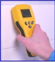
**Moisture Meter -Search Mode** The Protimeter MMS has a radio frequency moisture sensor located in a bulge at the top of the instrument. This is held against a surface to obtain a relative qualitative indication of the moisture level within the material / beneath the surface. In this way the user can establish if there are high moisture levels within material that warrant more detailed investigation. This technique is fast and does not mark or damage surfaces.
