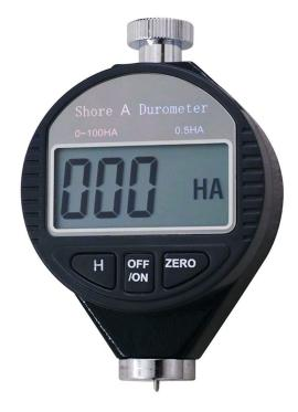
The SH-A Shore A digital rubber hardness tester is designed for testing the hardness of soft rubber, printer rollers and other elastomer materials (ASTM--D--2240). This easy to use hardness tester with simple structure and small body us lightweight and gives intuitive readings. Taking hand-held measurements and can also be placed in a cradle with a set load test.
