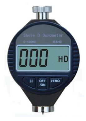
Shore digital rubber hardness tester is designed for testing the hardness of soft rubber, printer roller and other elastomer material (ASTM--D-2240). It has advantages of simple structure, convenient use, small body and light weight, intuitive readings. It can carry the hand-held measurements and can also be installed on the same type of fixed cradle which is matched with the set load test.
