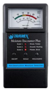
The MEP Moisture Encounter Plus detects and evaluates moisture conditions within various building materials by nondestructively measuring the electrical impedance.
