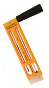
These instruments are designed to determine the dewpoint and relative humidity at any given time. The Elcometer 116A Whirling Hygrometer is available in Celsius scale. A guide for Relative Humidity (RH) determination is supplied with each instrument and the dewpoint can accurately be obtained using the Elcometer 114 Dewpoint Calculator.
