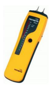
The Mini 2000 is probably the most widely used moisture meters in the world. These compact, general purpose moisture meters are used by building professionals and trades across the globe, to check the moisture level of wood and masonry products for a vast range of quality control and dampness diagnosis applications.
