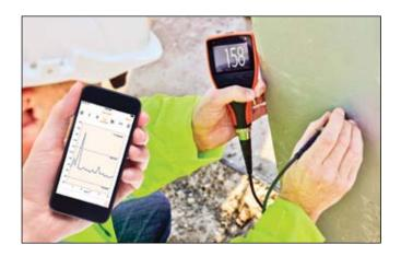
The ElcoMaster® Mobile App brings the office to where you are. You can connect Elcometer Bluetooth® enabled inspection gauges directly to iPhone, iPad and iPods or Android™ mobile phones and tablets via ElcoMaster® Mobile App.
