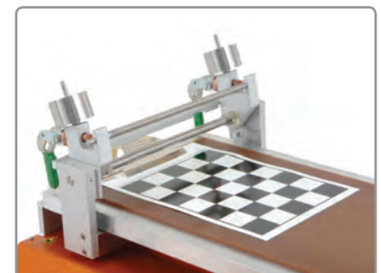
11 pre-set speeds and adjustable stroke length - from 5-150mm (0.2 - 5.9")
