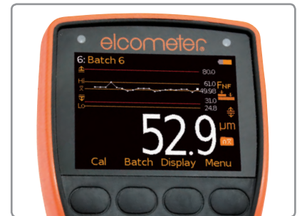
On-screen trend graph displaying last 20 measurement values
