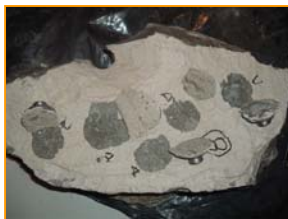
Adhesion testing of liners.
