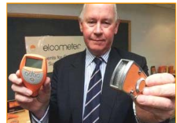
The digital Elcometer 456 (left) developed from the original "Elcometer" (now 101), which had no electrical parts.
