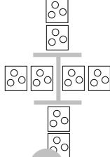
**Beams** (left) have two Reference Areas per metre length, both on the web (middle part) and on the flanges (top
