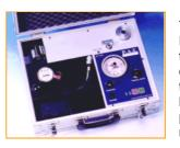
The Elcometer 110 and Elcometer 1920 adhesion testers provide а controlled increase in tension up to the breakpoint. These test parameters make the results more repeatable.
