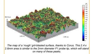
The way to decide if a special calibration should be done is to conduct a test. Measure some known thicknesses of plastic or known coated samples and determine the deviation. The best method and the gauge to use will depend on the job requirements and what functions are available in a particular model.
