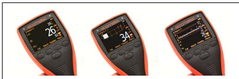
Put simply the user can now simply 'drag' the probe continuously across a coated surface and, upon removing the probe from the surface, at a glance, view the display to see the average, highest and lowest readings, as well as whether they are inside or outside any
