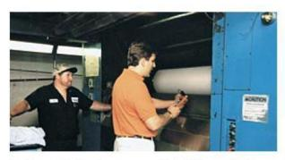
Joe demonstrating how to measure press blanket thickness using the Elcometer 355 at The Oakland Press in the 1990s.
