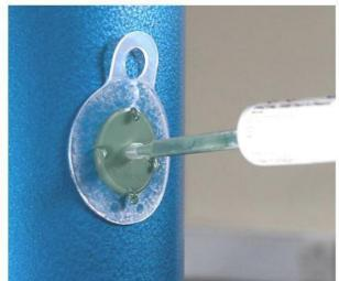
Once abraded, the ElcoPatch™ is placed over the abraded area (the patch has the same diameter as the abrasion ring). At this point, if required, the coating cartridge may be heated using Elcometer's cartridge heating system.
