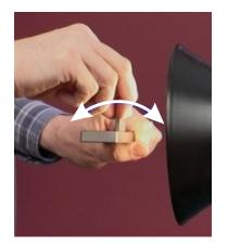
If light is visible, the scraper is not suitable for use and should be replaced.
