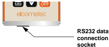
Figure 6. RS232 data connection socket
