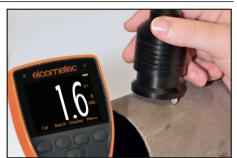
All Elcometer 224 Surface Profile Probes have an accuracy of  $\pm 5\%$  or  $\pm 5\mu$ m ( $\pm 0.2$ mil) and are supplied with a glass zero plate, calibration test foils; nominal values 125µm (5.0mils) & 508µm (20mils) and an Elcometer test certificate.
